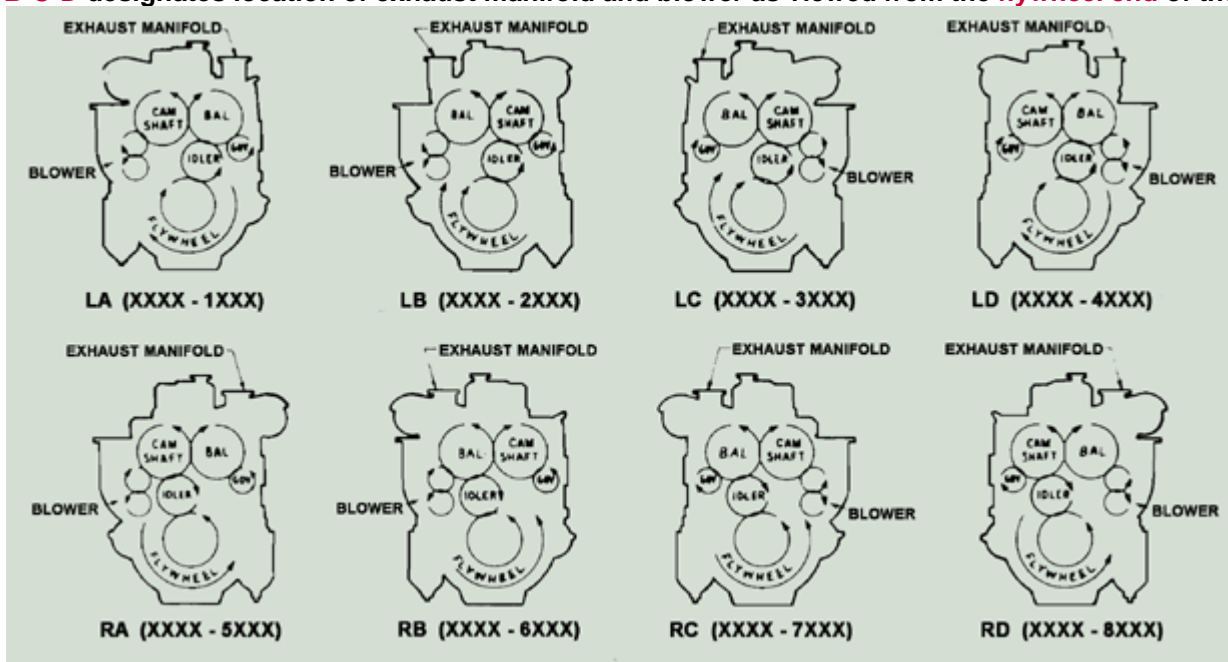
ALL VIEWS FROM REAR (FLYWHEEL) END OF ENGINE
