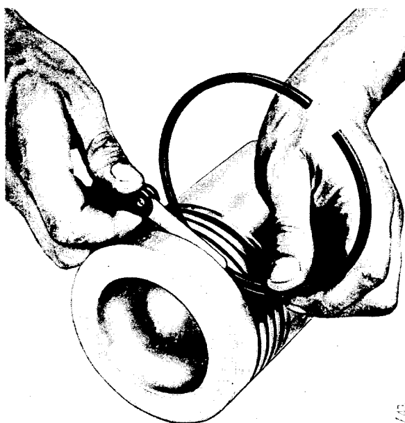
Fig. 7 Measuring axial play for piston ring
