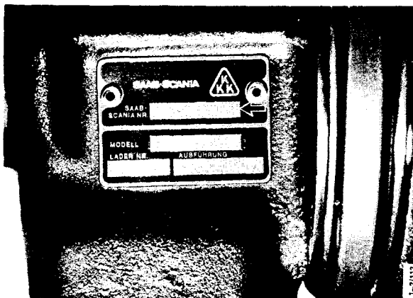
Fig. 2 Make KKK type 4LGZ. The Scania article number is stamped in where the arrow points. Fitted on engines for L trucks and on separate engines
