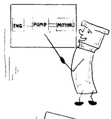
"To begin the transfer of power from an engine to the load, my pump takes the mechanical power of the engine and converts it to hydraulic power. Oil conveys the hydraulic power to my motor and it converts the hydraulic power back to mechanical for the output shaft!"
