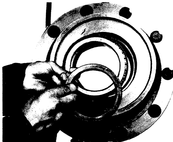
11. Inspect wheel bearings, cups and seal. Replace if necessary.
