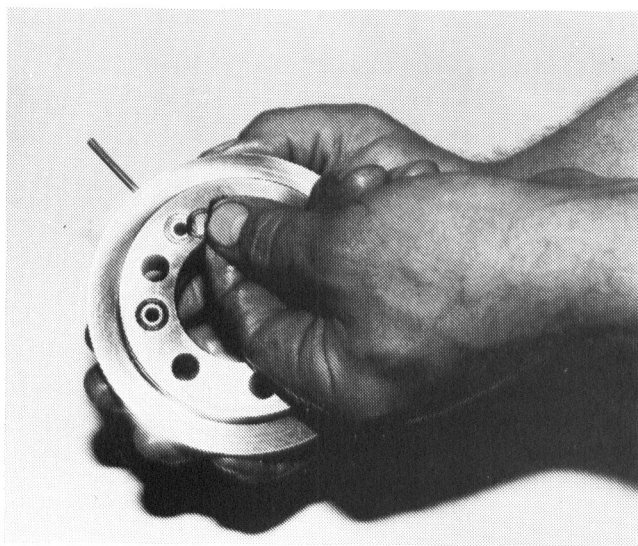
6. Insert both oil passage O-rings into grooves on inboard face of wheel retainer. Use a small amount of petroleum jelly to hold them in place and facilitate assembly.
