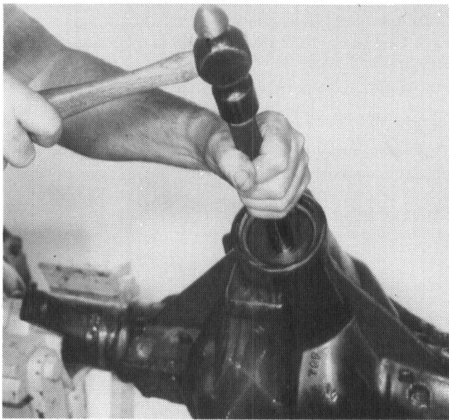
3. Assemble the outer pinion bearing cup into carrier as shown.
