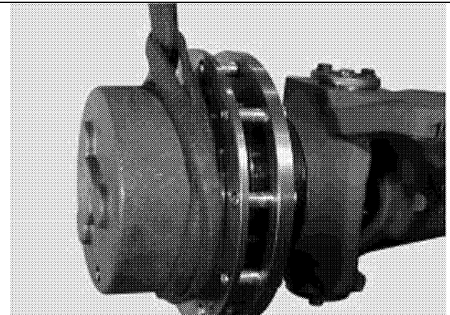
6m. Apply Loctite 515 on face of hub and install drive flange assembly. See Assembly Instruction Note #12.
