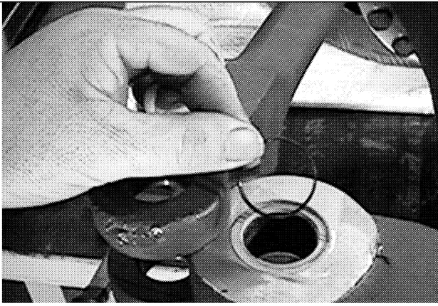
1l. Install new O-rings in clevis bore.
