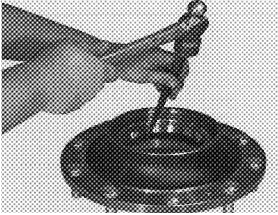
19b. Remove inner and outer bearing cups.
