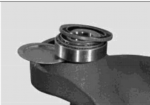
21j. Install grease retainers, cups, cones and seals.
