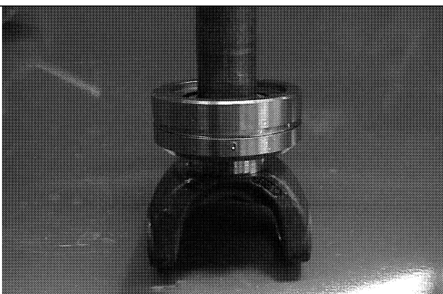
9. Install bearing retainer assembly on axle shaft with large chamfer facing yoke.
