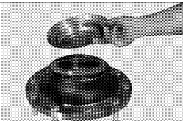
2i. Install new hub seal using proper driver. See Assembly Instruction Note # 11.
