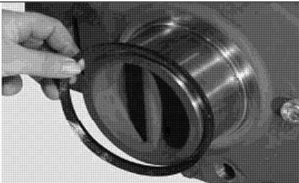
3d. Remove front trunnion grease seal. Inspect trunnion bushing and O-rings for damage. Remove and discard if damaged.
