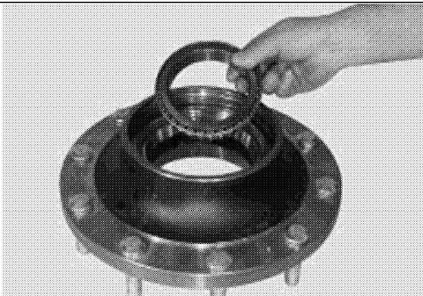
1i. Install new inner and outer bearing cups, and inner bearing cone in hub.
