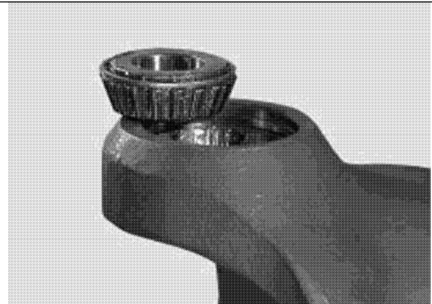
23j. Apply grease to cups and cones prior to installation.
