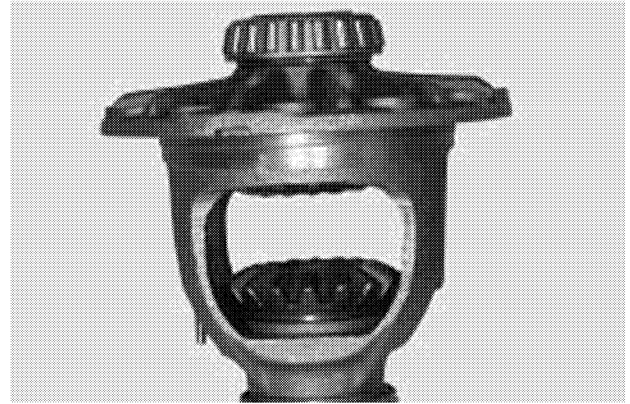
15g. Side gears and thrust washers installed.
