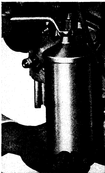
Fig. 17. Unscrewing the Oil Filter Bowl Securing Bolt.
