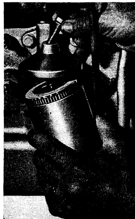
Fig. 18. Oil Filter with Filter Element Bowl Removed.
