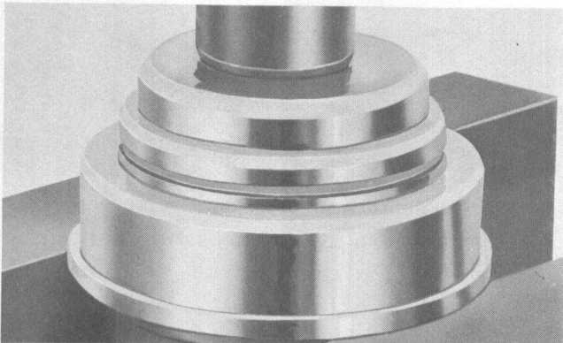
J. Remove the pinion quill rear bearing inner race using a suitable puller or press. Exercise care not to damage inner retainer against which race is assembled.
