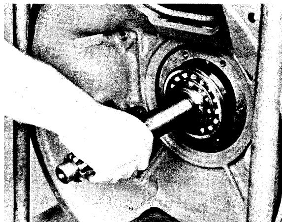
61. Installing drive gear assembly into case bore. Make sure pilot bearing on mainshaft seats properly in pocket of drive gear.
