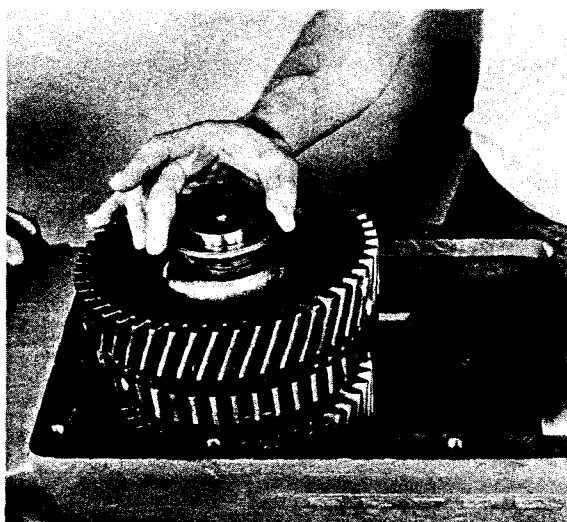
39. Installing washer on front of countershaft.
