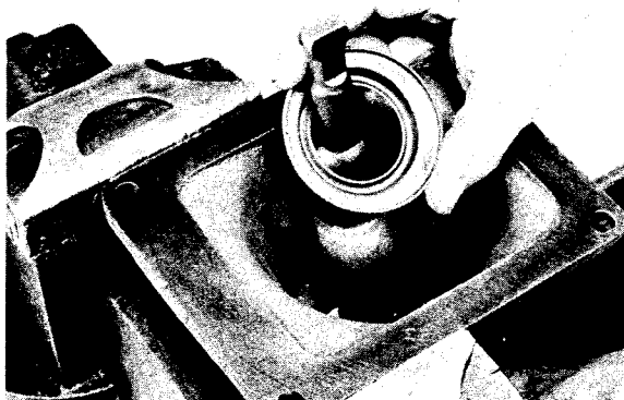
3. Removing washer and gear shift lever from housing.
