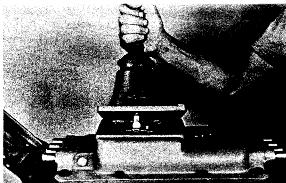
1. Removing the gear shift lever housing assembly.
