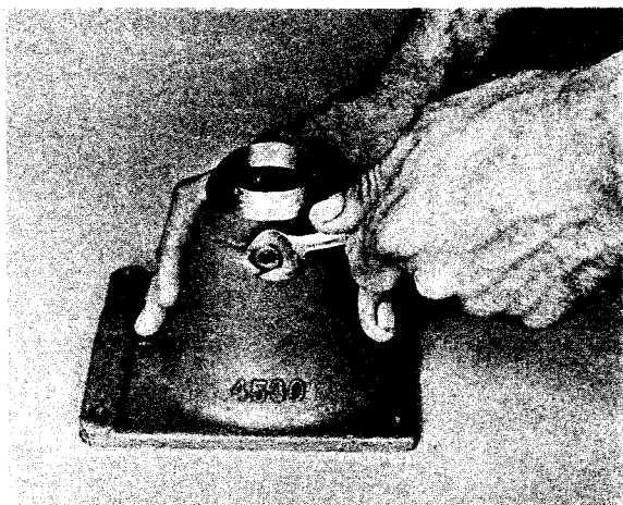
79. Installing lockwasher and nut on gear shift lever pivot pin.
