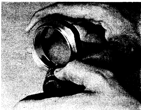
58. Applying Loctite to threads of drive gear bearing nut.
