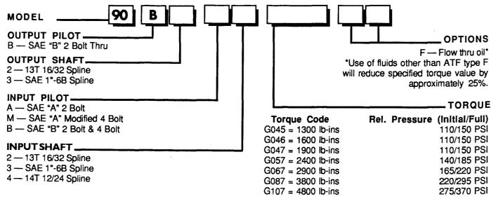
Torques listed are wet and at (0) PSI back pressure. Release pressures shown are minimum.
