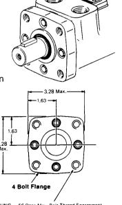
3/8-16 UNC x .56 Deep Max, Bolt Thread Engagement (4) Mounting Holes Equally Spaced on 3.25 Dia. Bolt Circle
