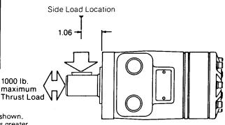
This chart is based on the load being applied at the location shown. Side load capacity decreases when load is applied at distances greater than shown.
