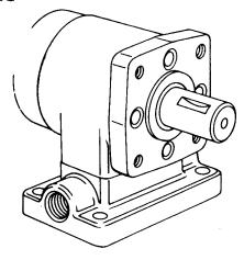
BASE BLOCK with Four Hole Flange
