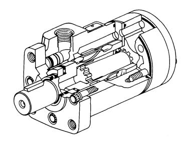
ounce than many units do per pound. This is possible because its power output is at slow speeds which can be matched to the application without belts, chains, or gear reductions.
