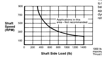
The side load capacity is more than adequate to handle any externally applied loads such as belts, chains, etc., as long as the motor is applied within its torque rating. The hydrodynamic bearing has long life when load ratings are not exceeded.
