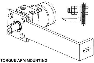
This is a simple, easily made mount and when properly designed and installed, it will compensate for shaft misalignment. The torque arm should be at least 8 inches long to prevent excessive side load. Install on the machine as shown in the inset. This allows for both lateral and longitudinal play and still holds the motor steady with minimum side load.
