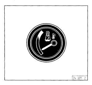
■ The pointer of the engine temperature indicator must always be in the green sector – in the yellow-green area as an exception only. If the pointer moves to the orange sector, the engine is becoming too hot. Stop the engine and trace the trouble cause with the aid of the Diagnosis Chart (see 7.1).
