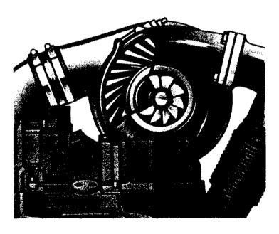
The overall efficiency of the Forward Plan turbo was raised by reshaping the compressor wheel blades.
