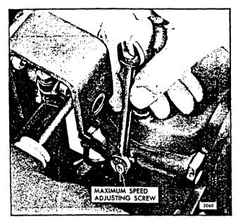
Fig. 5 - Adjusting Maximum Engine Speed
