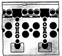
Severe thermal shock testing proved the extreme crack resistance of the new design. In the test, the engine was run at excessive horse-power for a minute and a half, then shut off with the cylinder head very hot. Cool water was circulated during the shutdown for a minute and a half, then the engine was started again, run another minute and a half, and so on. As shown, the standard
