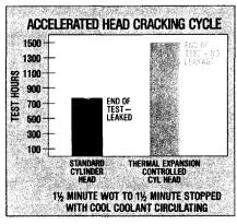
cylinder head cracked within 750 hours. With the thermal expansion head there was no leakage at 1500 hours where the test was ended. The test shows the thermal expansion head to be much more tolerant to user abuse or accidental overheating.
