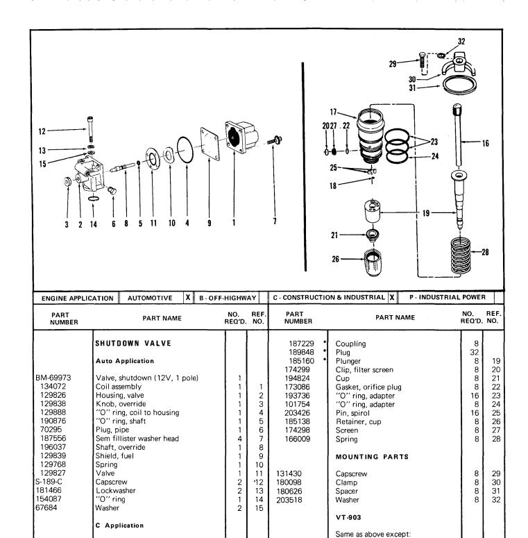
Link, injector 8 AR-40026 16 Barrel and plunger Injector, less link 8 17 Adapter 8 Note: Not sold separately. Barrel and plunger 8 Ball, check 8 18 Barrel 8 19
