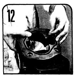
Grease the new gasket seals and insert them into the grooves in both sides of all gear housings. Position the first gear housing over the shaft end cover and dowels. Tap it with a soft hammer until it rests tightly against the shaft end cover. Be careful not to pinch the gasket seal. Also be sure the large rounded core is on the inlet side.
