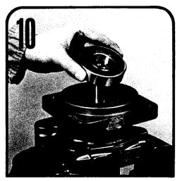
If the unit is equipped with an outboard bearing, guide the bearing into its recess in the shaft end cover. This is a light press fit. It may be necessary to lightly tap the bearing into the bore.
