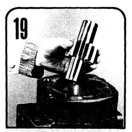
Place the thrust plate in the gear housing per Step #14. Insert the drive and driven gears of the second section in their respective bearings. Make certain gears are in contact with thrust plate face. Place the port end cover plate in the housing per Step #16.
