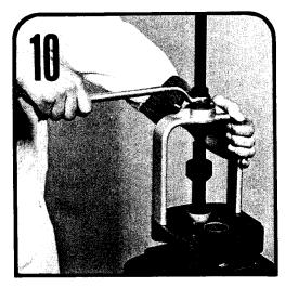
Inspect all bushings for scoring or discoloration and replace if necessary. Use a bushing puller as shown in the tool list to remove bushings (see page 12).
