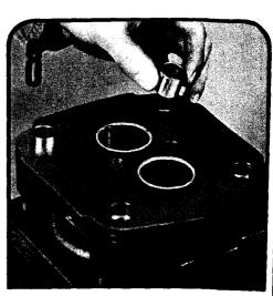
See that dowel pins are in place in any new castings. Examine all dowels. (See page 12). Before inserting make certain the hole is clean and free from burrs. Gently start pin straight into hole and tap lightly with a soft hammer.
