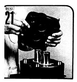
Place the port end cover over the gear journals. Align the dowels with the holes in the mating casting. Being careful not to pinch the gasket seal, tap the port end cover lightly in the center between bearing bores to engage the dowels and to move parts together in final seating.
