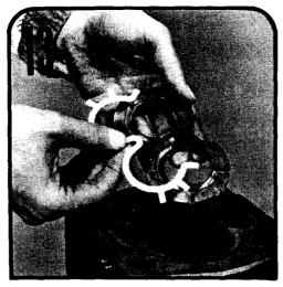
Assemble the channel seals into the grooves in the thrust plates with the flat side of the seal facing away from the thrust plate as shown below.
