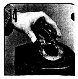
Gently slip the thrust plate through the gear housing and into place on the shaft end cover. The channel seal from Step #13 should face the shaft end cover. The relief groove in the plate should face the outlet side of the pump.
