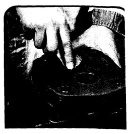
If bushings have been removed, deburr the bushing bores with emery cloth. Rinse parts in a solvent. Air blast all parts and wipe with a clean lintless cloth before starting assembly.
