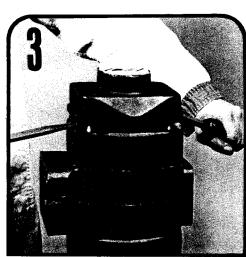
Lift off the port end cover. If prying is necessary, be careful not to damage the machined surfaces. Dowel pins will remain in either port end cover or gear housing. **Do not remove.**
