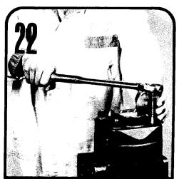
Thread the 4 fasteners (cap screws and washers, or studs, washers, and nuts) into the shaft end cover and tighten alternately or cross-corner. Rotate the drive shaft with a 6' wrench to make certain there is no binding in the pump. After the fasteners are tight and you are sure there is no internal binding, torque the diagonally opposite fasteners to 200 ft. lbs. (2400 in. lbs.), 140 ft. lbs. (1680 in. lbs.) for P315 models.
