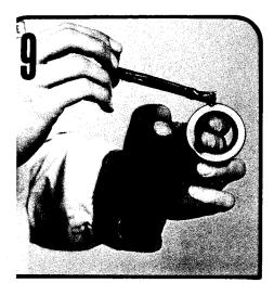
Before inserting a new lip seal in the shaft end cover, coat the outer edge of the lip seal and its recess with Permatex Aviation Form-A-Gasket No. 3 non-hardening sealant or equivalent. With the metal side of the lip seal up, press it into the mounting flange side of the shaft end cover with an arbor press and bar (see Tool List). Be careful not to damage the lip of the seal. Press in until flush with the recess. Wipe off excess sealant.
