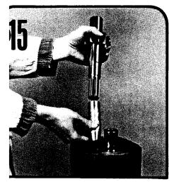
Slide the driven gear through the housing and into the bushing in the shaft end cover. Coat the steel sleeve tool with grease. Place the lightly greased drive shaft inside the sleeve and slide both through the shaft end cover with a twisting motion until the integral gear rests against the thrust plate. Avoid damaging the double lip seal. Remove the steel sleeve. Squirt clean oil over the gears.
