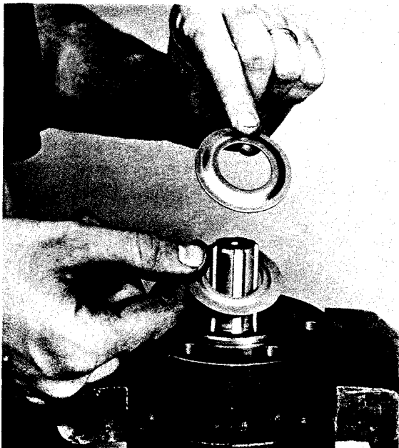
Fig. 24 Installing bearing seal and shield
