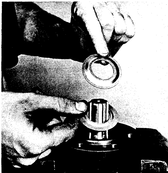
Fig. 8 Installing bearing seal and shield
