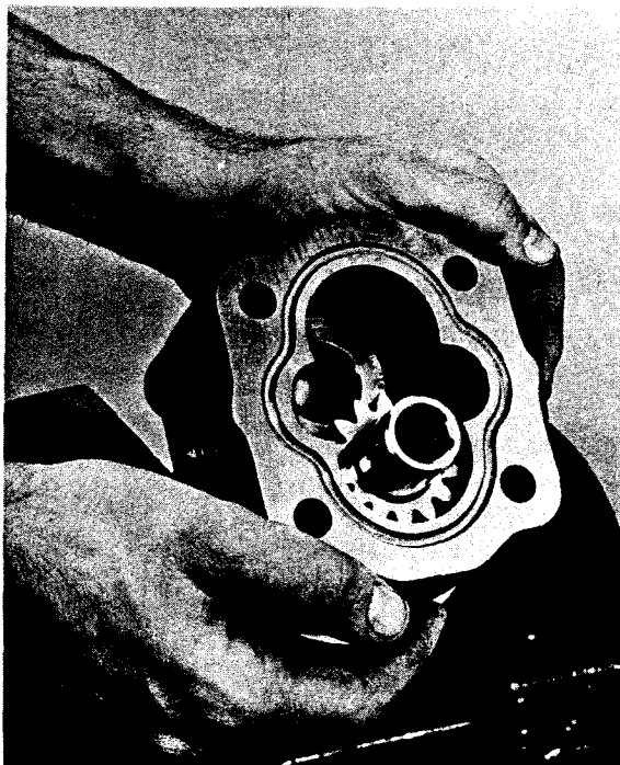
Fig. 15 Installing gear housing
