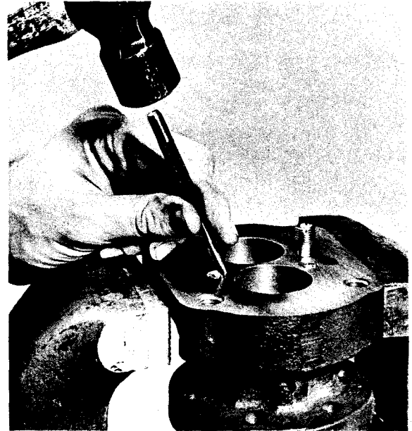
Fig. 21 Peening over check valve seat
