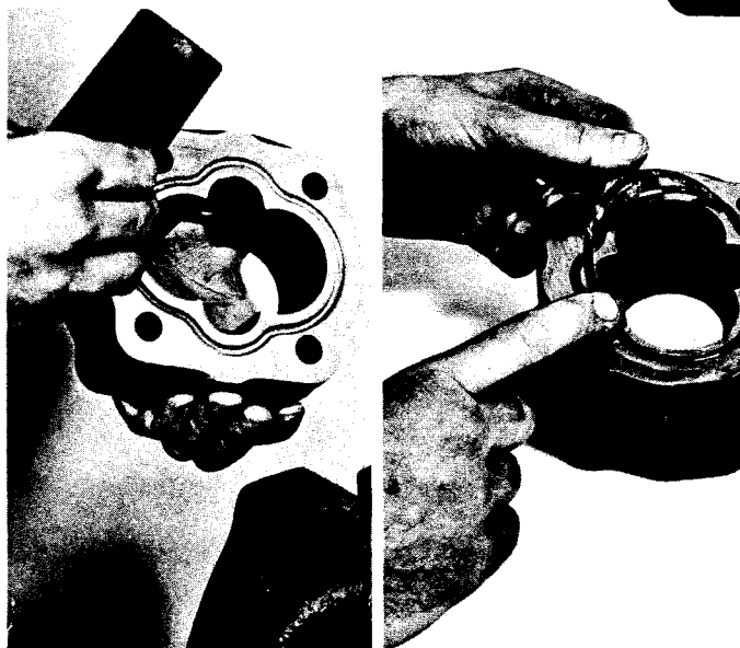
Fig. 29 Installing pre-greased "O" ring
