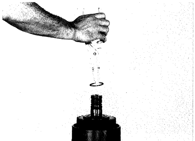
Figure 169 Remove clutch gear outer bearing retainer ring.
