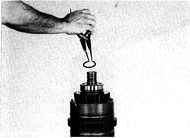
Figure 104 Remove front bearing retainer ring.
