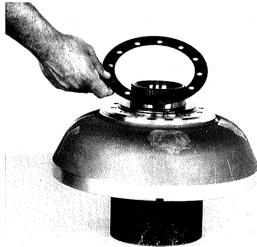
Figure 286 Position backing ring on impeller.
