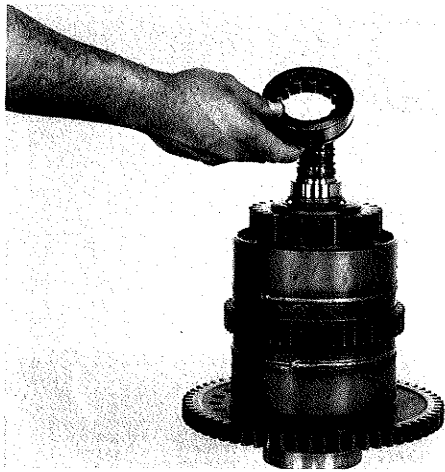
Figure 158 Position front bearing over bearing race.
