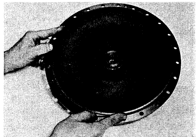
Figure 160 Install a new impeller cover "O" ring and grease lightly to facilitate reassembly.
