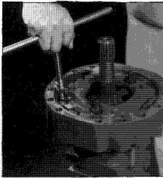
ASSEMBLARE IL SPINGIDISCO CON I PUNTALINI VERTICALI.
