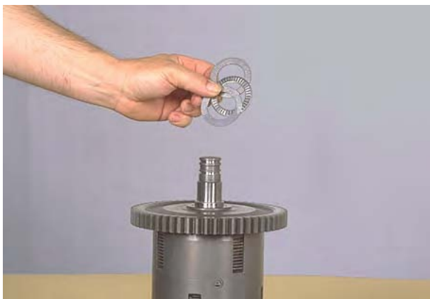
Figure 61 Remove outer thrust washer, bearing and inner thrust washer.
