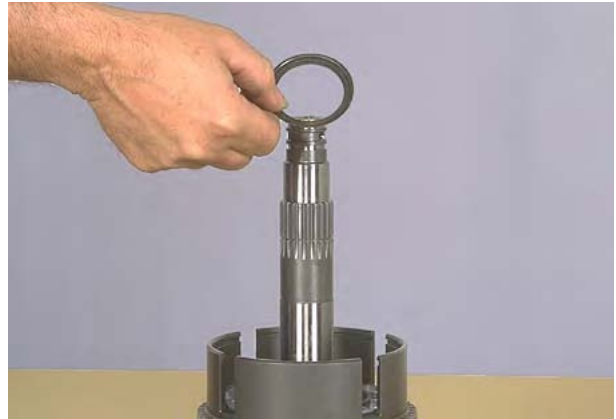
Figure 151 Remove retainer ring retainer.
