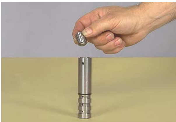
Figure 12 Remove accumulator spool. Ref. figure 8.
