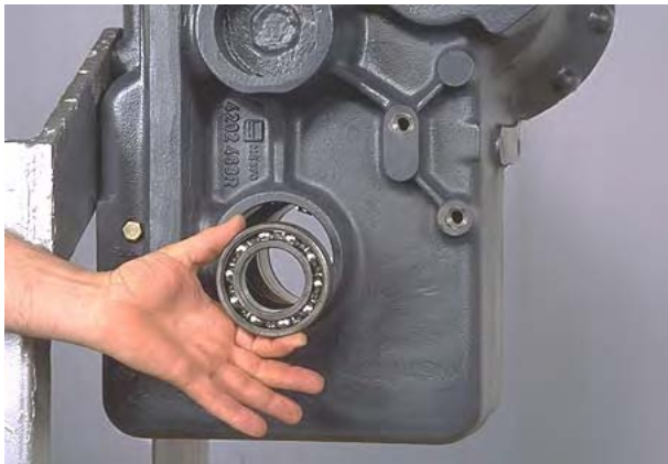
Figure 44 Remove output shaft rear bearing.
