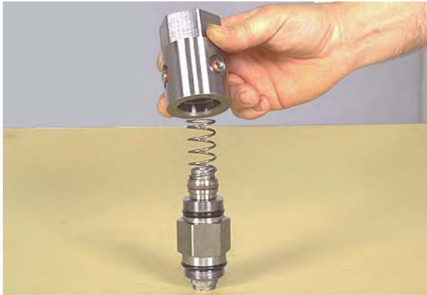
Figure 28 Remove hydraulic inching cover.
