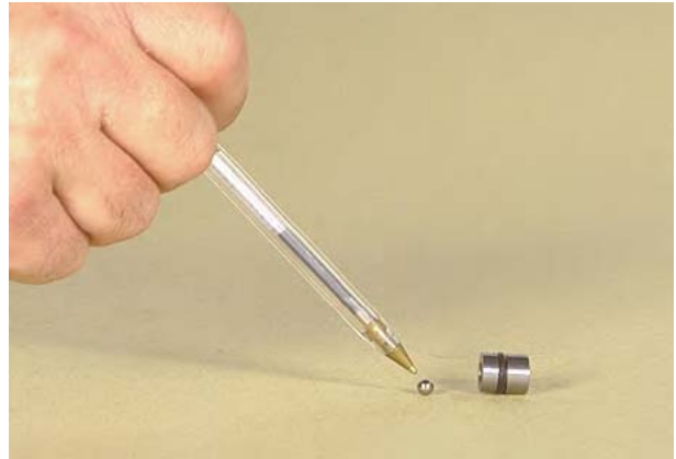
Figure 19 Remove check ball.
