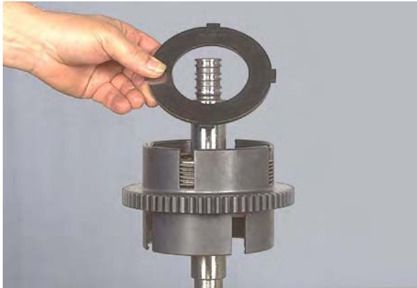
Figure 232 Remove end plate.
