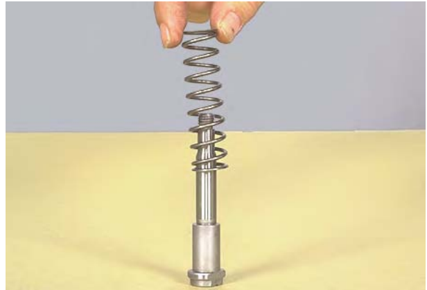
Figure 37 Remove inching return spring.
