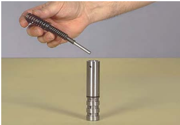
Figure 11 Remove modulator valve outer, middle and inner springs and spring stop ref. figure 7.
