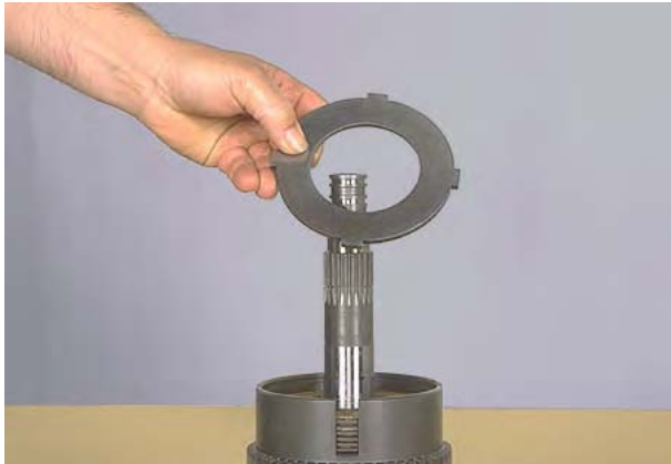
Figure 148 Remove end plate.
