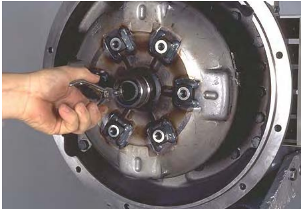
Figure 422 Install converter assembly retainer ring.
