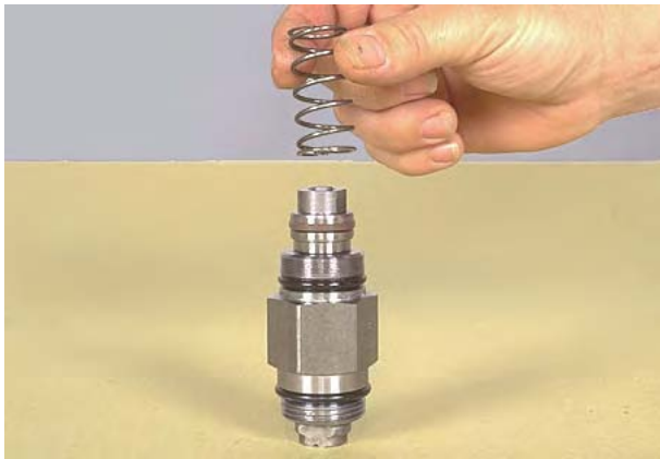
Figure 29 Remove inching return spring.
