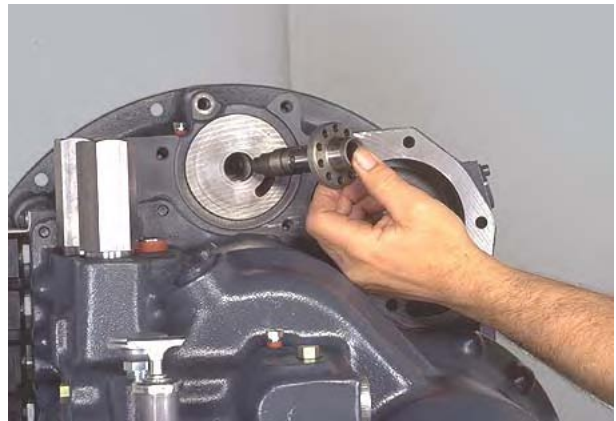
Figure 426 Install regulator sleeve assembly in converter housing.
