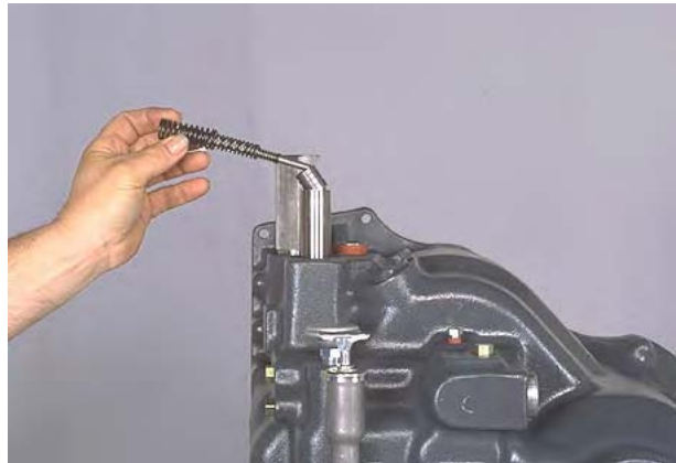
Figure 47 Remove inner, middle and outer springs. Remove valve stop pin and accumulator spool. Remove regulator spool and sleeve assembly.
