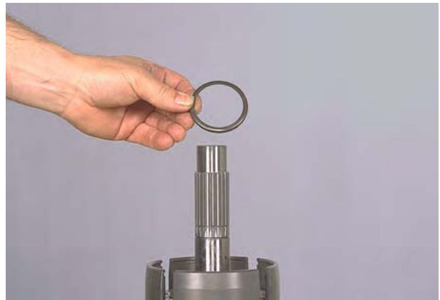
Figure 90 Remove clutch piston wear plate.
