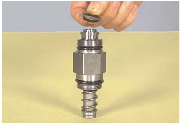
Figure 32 Remove hydraulic piston seal.
