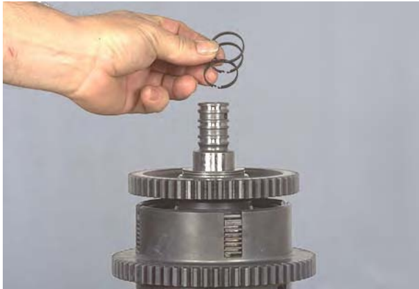
Figure 226 Remove clutch shaft oil sealing rings.
