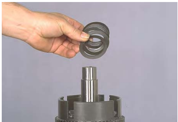
Figure 166 Remove disc springs. NOTE: See page 10-85.
