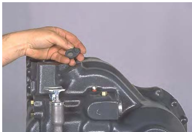
Figure 48 Remove sensor hole plug and "O"-ring.
