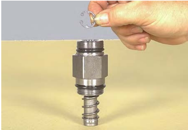
Figure 34 Remove snap ring.
