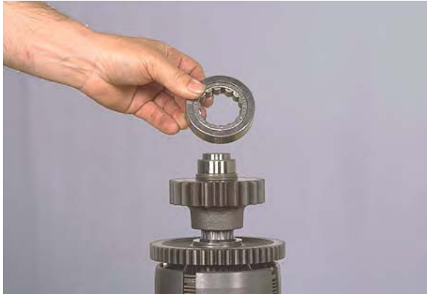
Figure 74 Remove clutch shaft rear bearing outer race.
