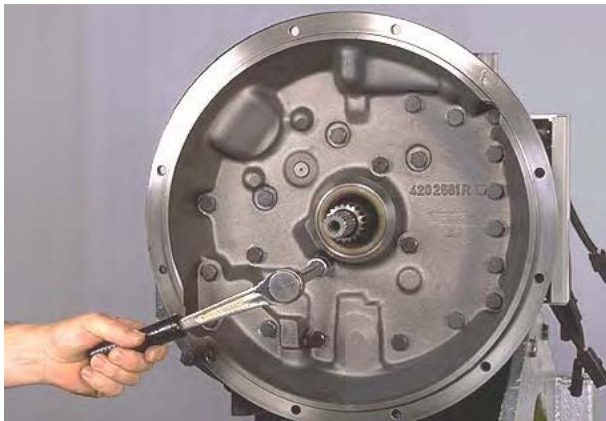
Figure 14 Remove converter housing to transmission case bolts and washers.
