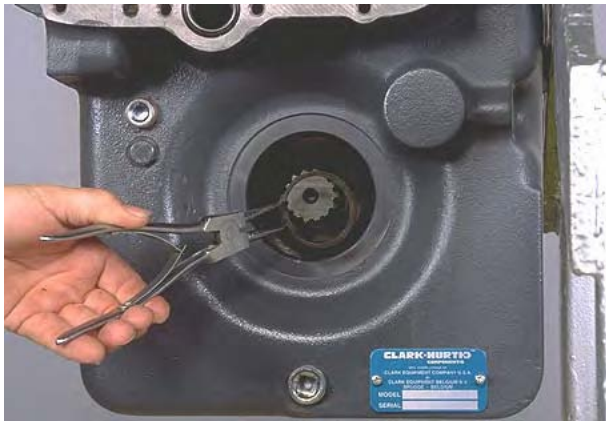
Figure 38 Remove output gear to shaft retainer ring.
