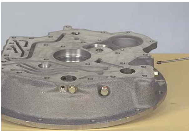
Figure 361 Remove oil distributor sleeve set screw.
