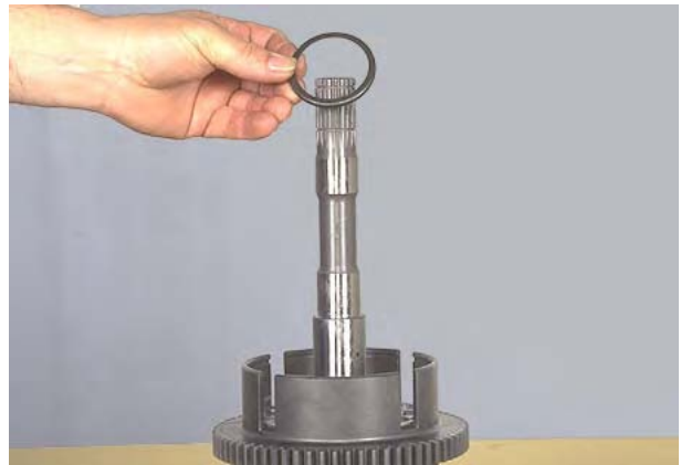
Figure 224 Remove clutch piston wear plate.
