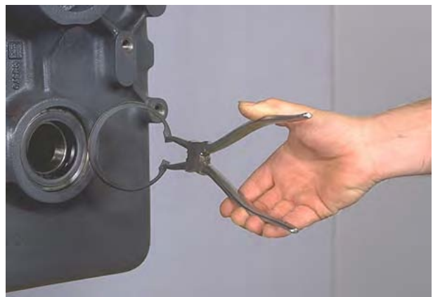
Figure 42 Remove flange oil seal sleeve retainer ring.
