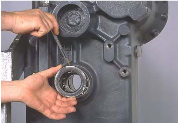
Figure 43 Remove sleeve and "O"-ring.
