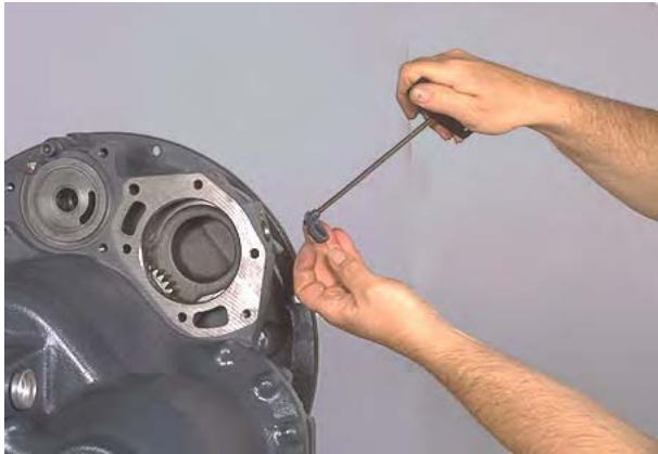
Figure 13 Remove sensor port plug and "O"-ring.
