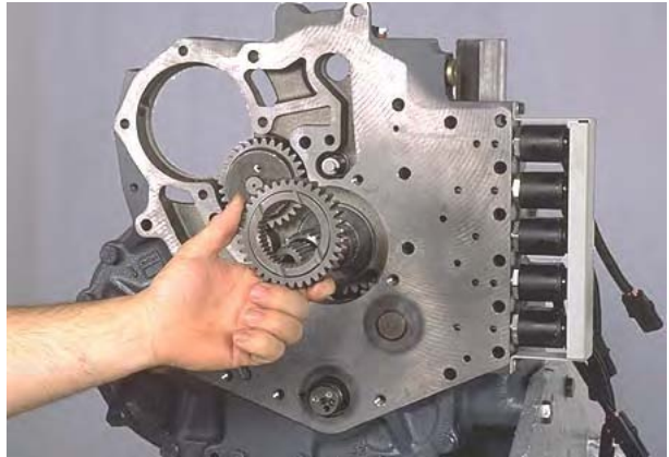
Figure 16 Remove impeller hub gear.
