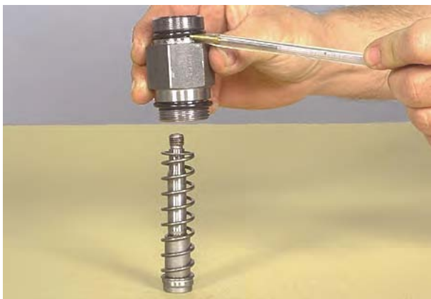
Figure 36 Remove hydraulic inching body and "O"-rings.
