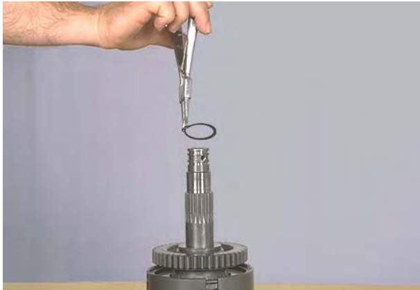
Figure 142 Remove outer thrust washer retainer ring.
