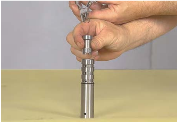
Figure 16 Remove regulator spool sleeve retainer ring.
