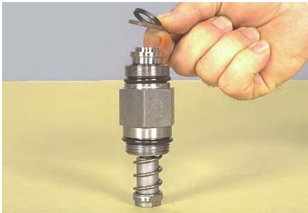
Figure 44 Install hydraulic piston seal.
