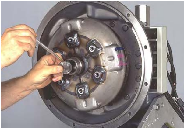
Figure 423 With new "O"-ring in place, install bore plug in converter assembly.
