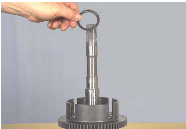
Figure 222 Remove retainer ring retainer.
