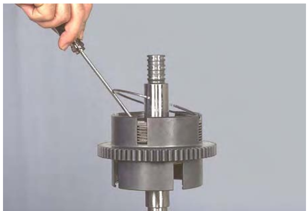
Figure 231 Remove end plate retainer ring.
