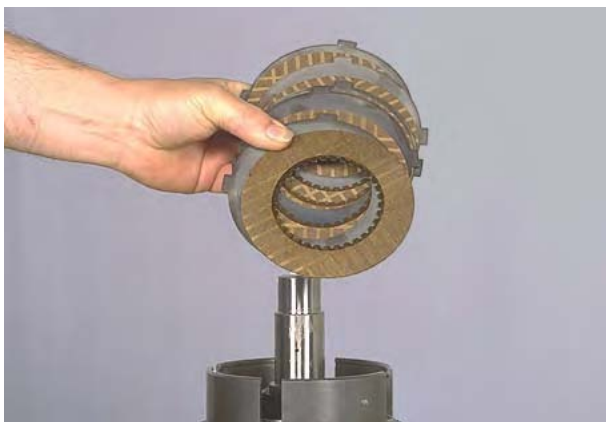
Figure 163 Remove clutch discs.
