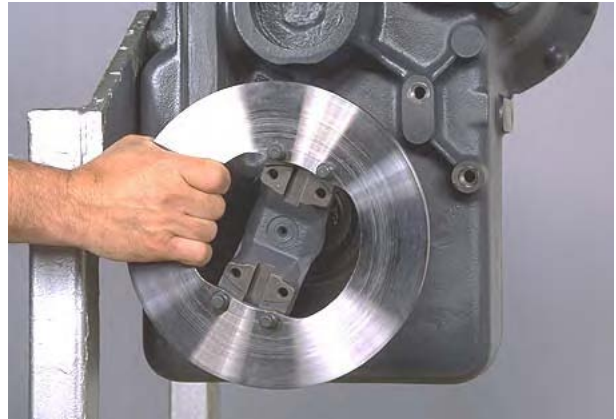
Figure 40 Flange removed. NOTE: brake disc is optional and was removed with flange.
