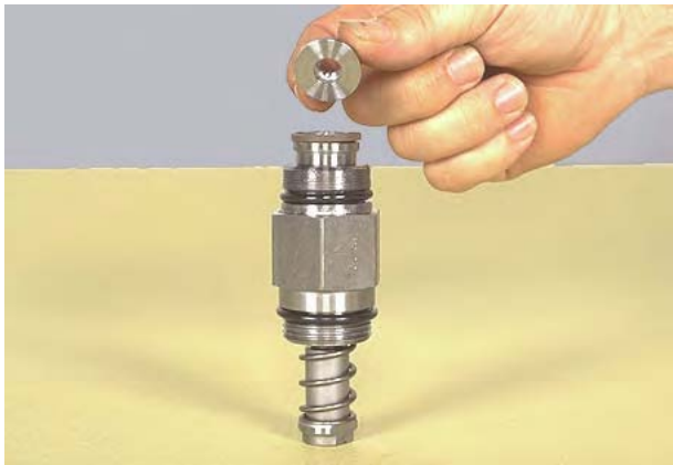
Figure 45 Apply Loctite nr. 243 to thread of inching actuator rod, install inching upper piston.
