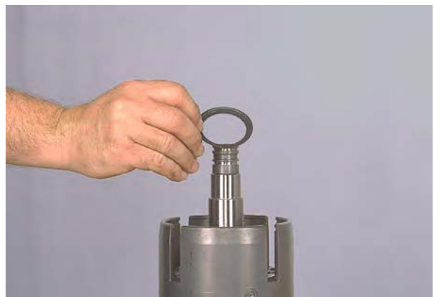
Figure 70 Remove retainer ring retainer.
