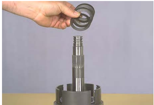
Figure 152 Remove disc springs. NOTE: see page 10-85.
