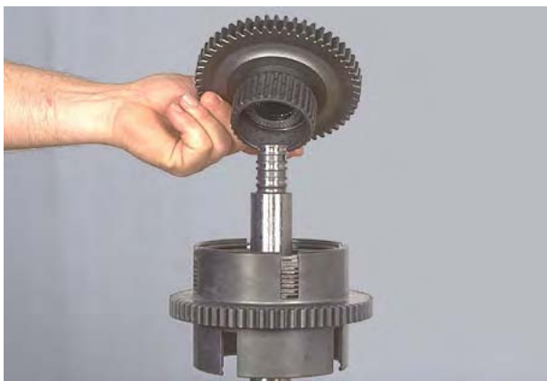
Figure 228 Remove clutch gear and disc hub.
