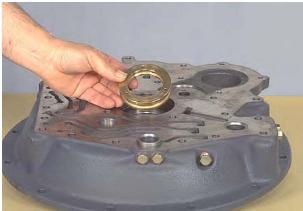
Figure 354 Remove oil distributor.
