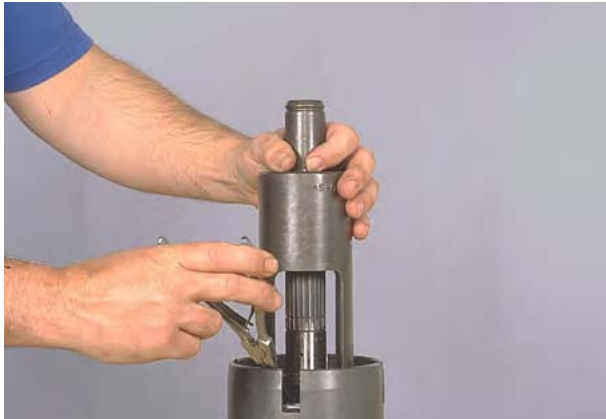
Figure 86 Compress disc springs and remove retainer ring.
