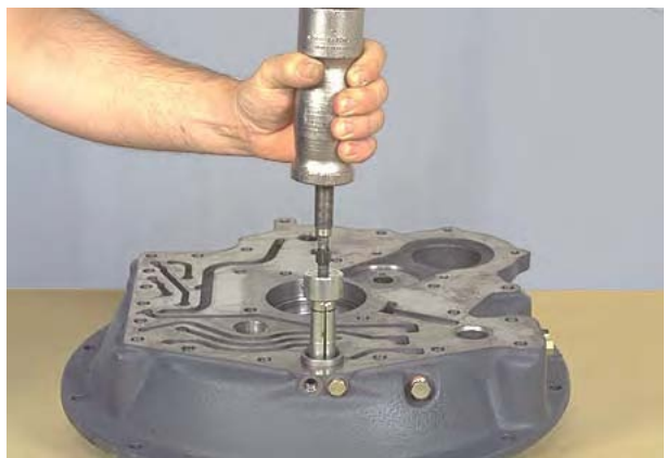
Figure 358 Using a hammer puller as shown, remove oil distributor sleeve (high and 3rd).
