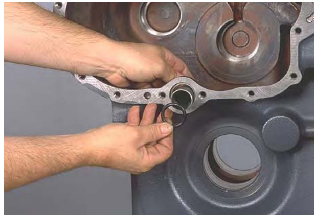
Figure 53 Remove supply tube "O"-ring.
