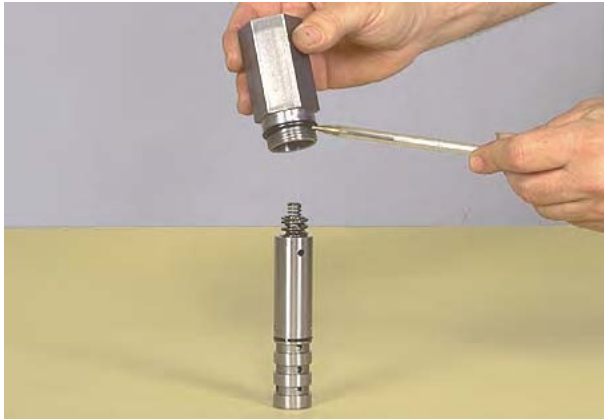
Figure 10 Remove modulator valve body "O"-ring.
