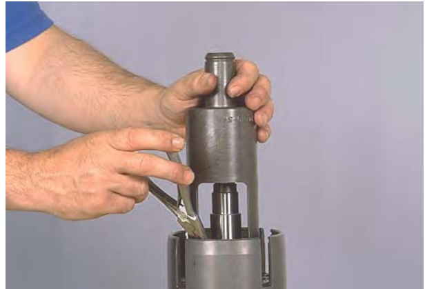
Figure 68 Compress disc springs and remove retainer ring.
