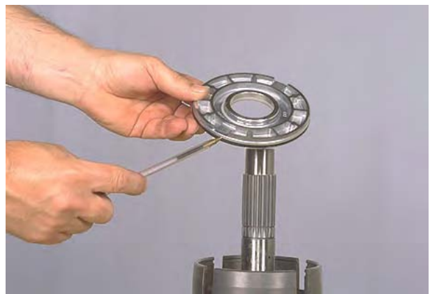
Figure 91 Remove clutch piston.
