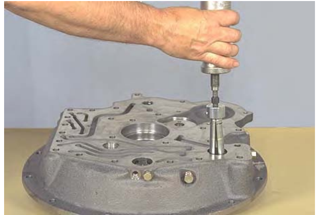
Figure 362 Using a hammer puller as shown, remove oil distributor sleeve (1st and 2nd).
