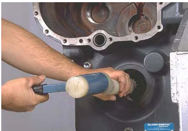
Figure 39 Tap output shaft and flange from housing.
