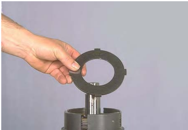
Figure 162 Remove end plate.
