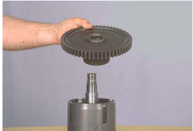
Figure 62 Remove clutch gear and disc hub.
