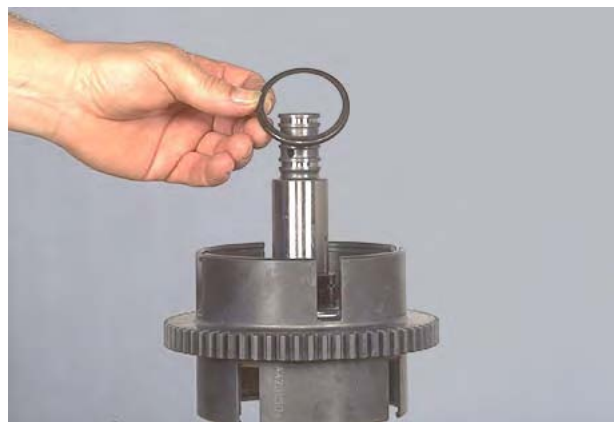
Figure 237 Remove clutch piston wear plate.
