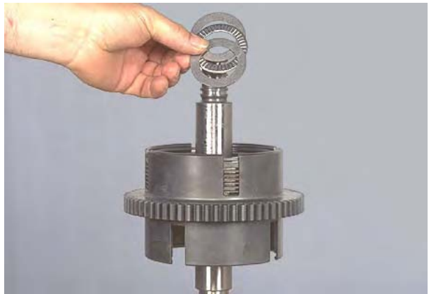
Figure 230 Remove outer thrust washer, thrust bearing and inner thrust washer.
