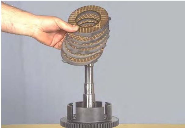
Figure 220 Remove clutch discs.
