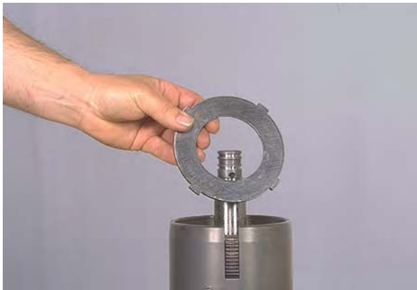
Figure 66 Remove clutch disc end plate.
