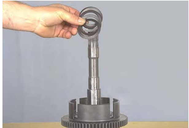
Figure 223 Remove disc springs. NOTE: see page 10-85.
