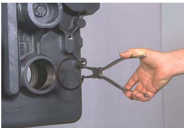
Figure 45 Remove bearing locating ring.
