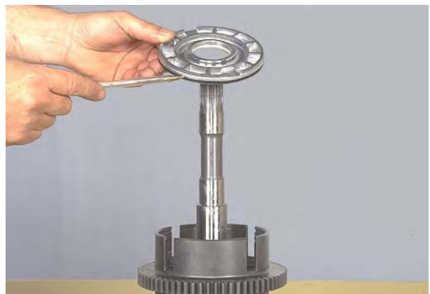
Figure 225 Remove clutch piston.
