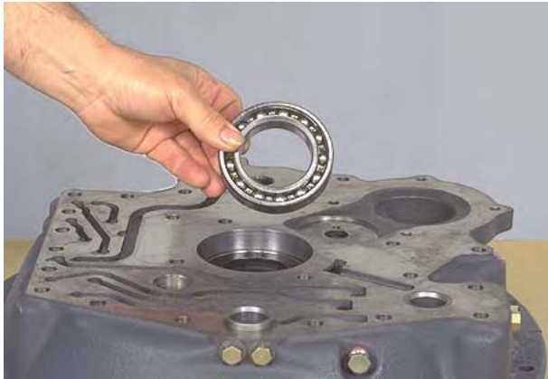
Figure 353 Remove torque converter bearing.
