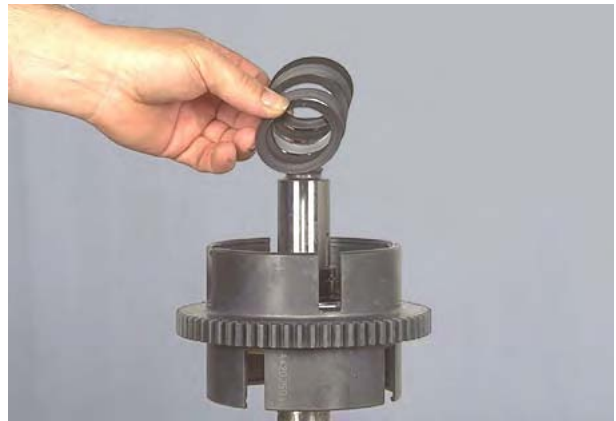
Figure 236 Remove disc springs. NOTE: see page 10-85.
