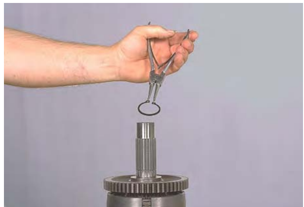
Figure 79 Remove thrust bearing and clutch gear retainer ring.
