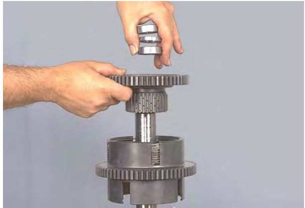
Figure 229 Remove bearings and spacer from clutch gear.
