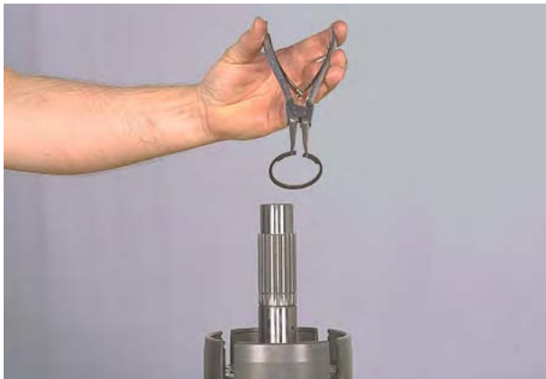
Figure 87 Remove retainer ring.
