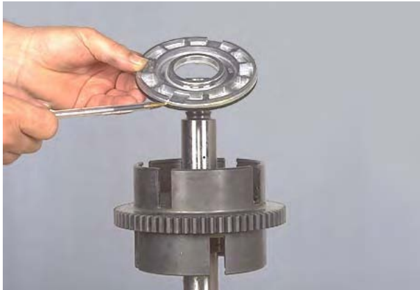
Figure 238 Remove clutch piston.
