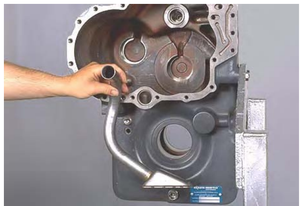
Figure 54 Remove supply tube and screen assembly.
