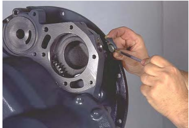
Figure 425 Install sensor hole plug end "O"-ring.
