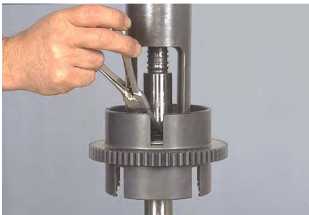
Figure 234 Compress disc springs and remove retainer ring.
