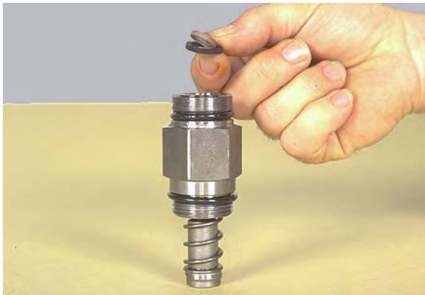
Figure 35 Remove hydraulic inching body seal.
