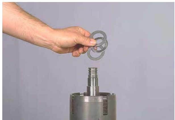
Figure 64 Remove outer thrust washer, thrust bearing and inner thrust washer.
