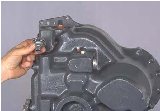
Figure 50 Remove air breather.
