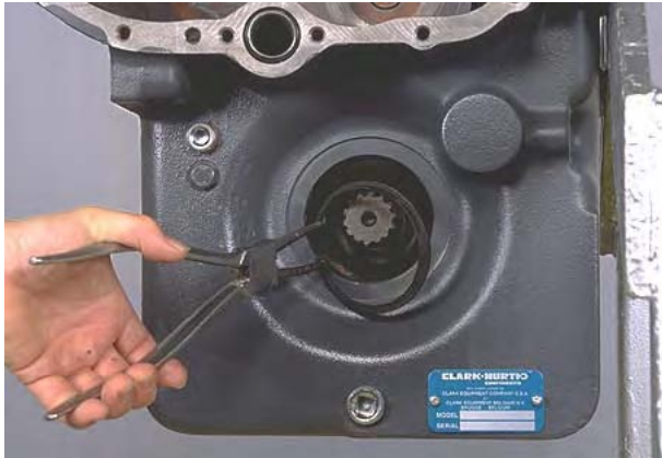
Figure 37 Remove bearing locating ring.
