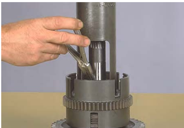
Figure 150 Compress disc springs and remove retainer ring.
