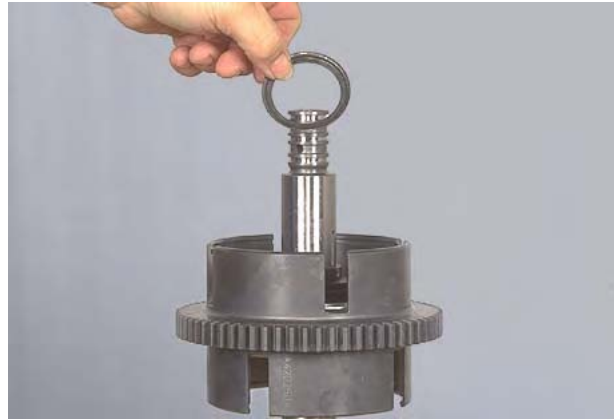
Figure 235 Remove retainer ring retainer.
