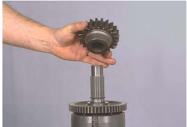
Figure 77 Remove gear from shaft.
