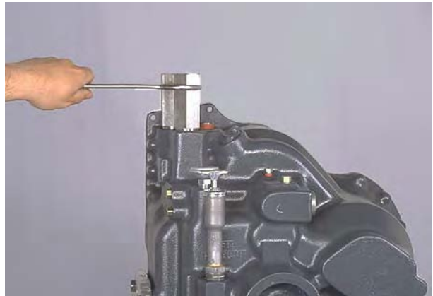
Figure 46 Remove modulator valve housing. NOTE: for single modulation and hydraulic inching. See section 11.1.
