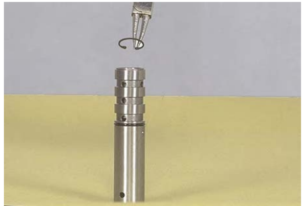
Figure 14 Remove regulator spool assembly retainer ring.
