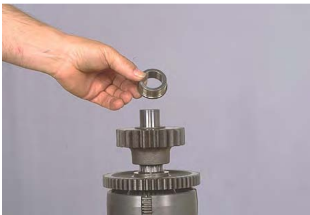
Figure 76 Remove inner race from shaft.
