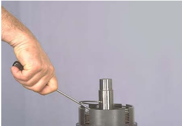
Figure 161 Remove end plate retainer ring.
