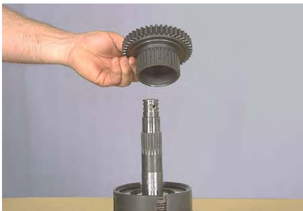
Figure 144 Remove clutch gear and disc hub.
