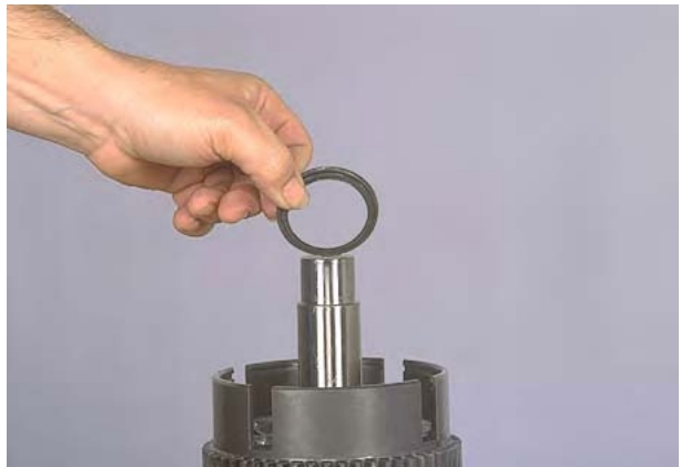
Figure 165 Remove retainer ring retainer.
