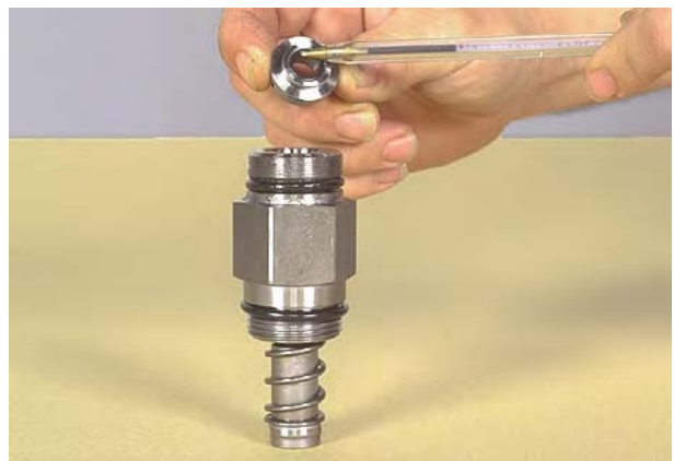
Figure 33 Remove inching lower piston and "O"-ring.
