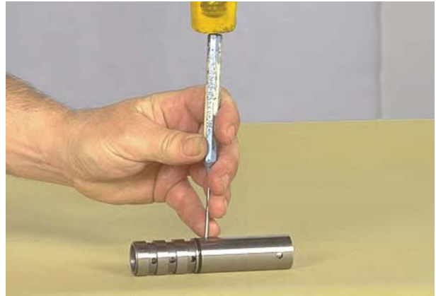
Figure 13 Remove modulator sleeve pin.
