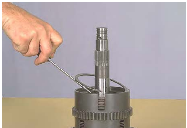
Figure 147 Remove end plate retainer ring.
