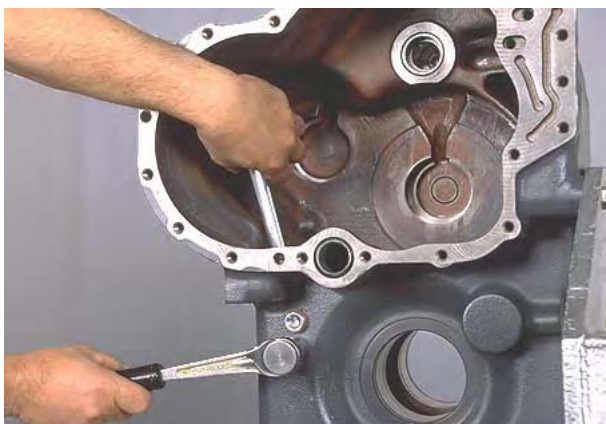
Figure 51 Remove supply tube retainer screw.
