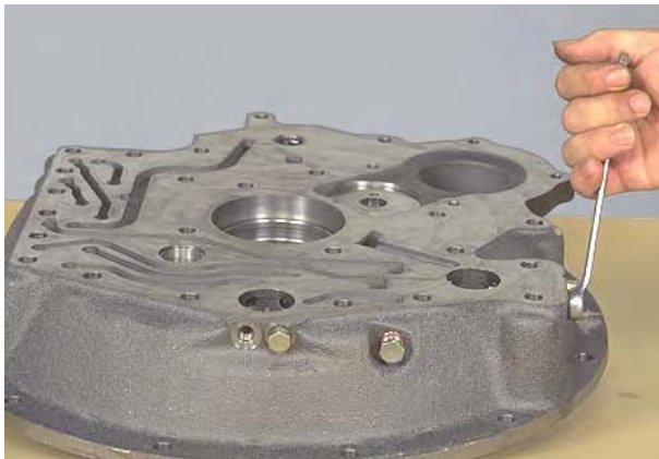
Figure 360 Remove converter housing plug (1st and 2nd clutch shaft).
