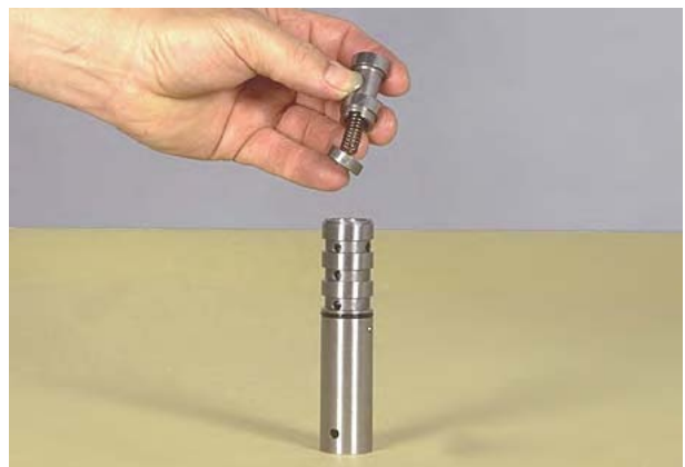
Figure 15 Remove regulator spool stop, spring and spring and sleeve assembly .
