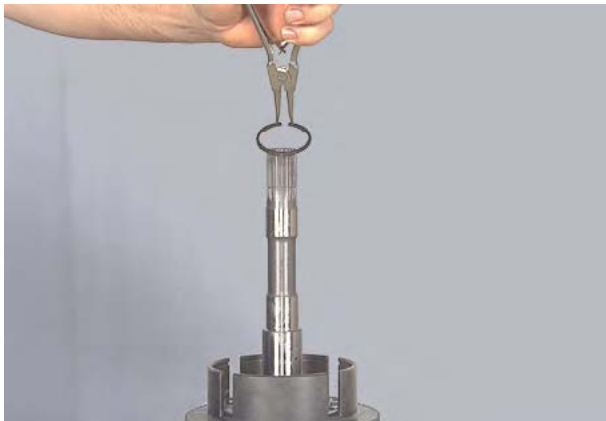
Figure 221 Compress disc springs and remove retainer ring.
