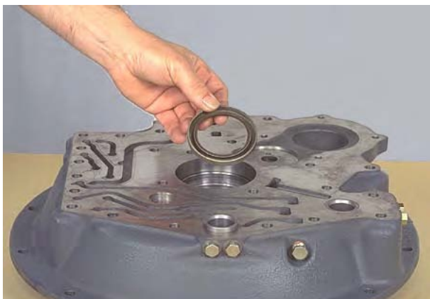
Figure 355 Remove converter oil seal.
