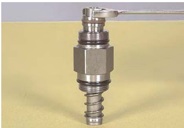
Figure 30 Remove hydraulic inching upper piston.
