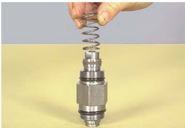
Figure 46 Install inching return spring.
