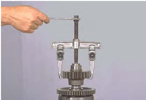
Figure 75 Using a gear puller as shown, remove gear and rear bearing inner race.
