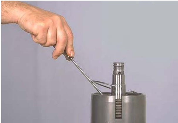
Figure 65 Remove clutch disc end plate retainer ring.
