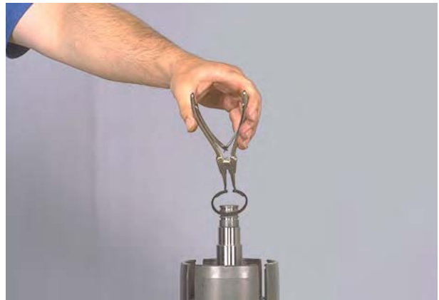
Figure 69 Remove retainer ring.
