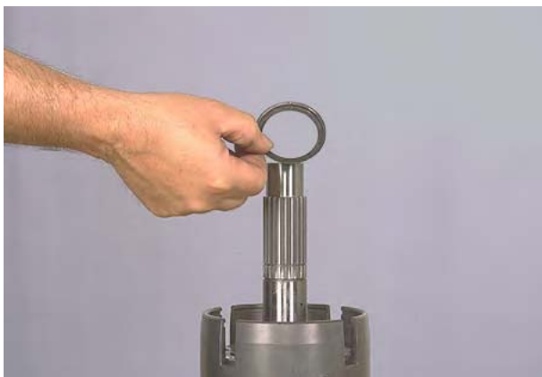
Figure 88 Remove retainer ring retainer.
