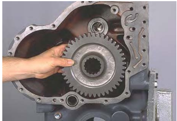
Figure 41 Remove output gear.
