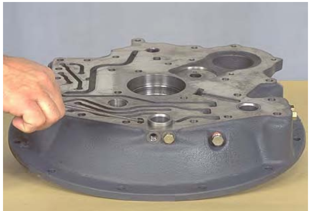
Figure 357 Remove oil distributor sleeve set screw.
