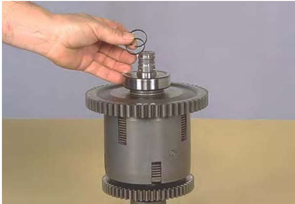
Figure 59 Remove clutch shaft oil sealing rings.
