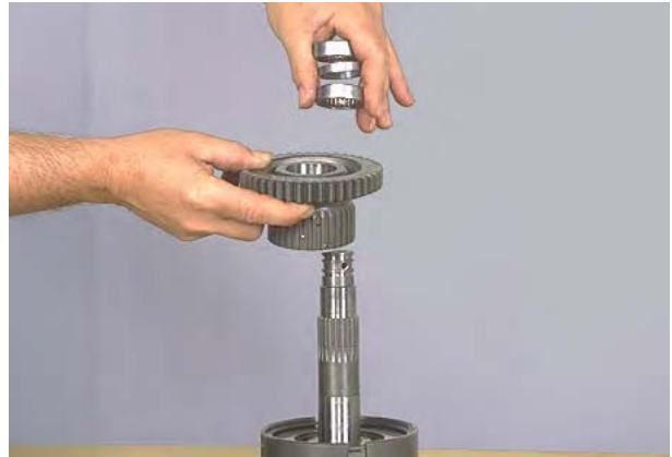
Figure 145 Remove bearings and spacer from clutch gear.
