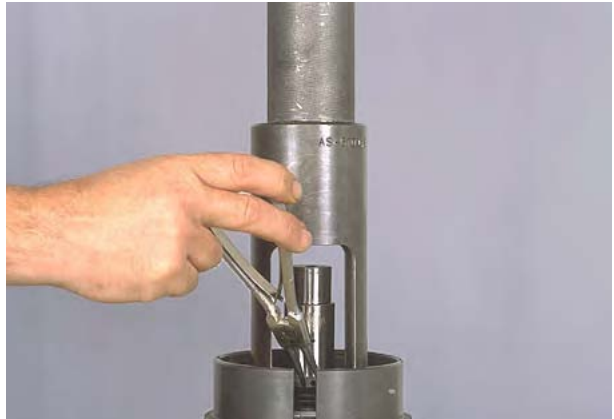
Figure 164 Compress disc springs and remove retainer ring.
