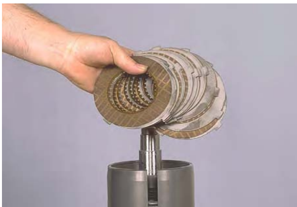
Figure 67 Remove inner and outer clutch discs.
