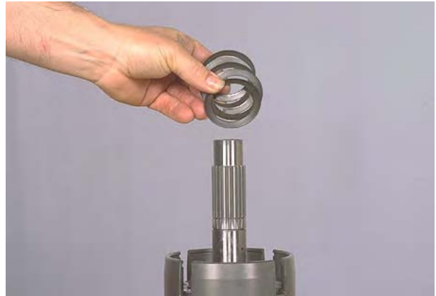
Figure 89 Remove disc springs. NOTE: see page 10-85.
