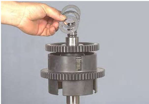
Figure 227 Remove outer thrust washer, thrust bearing and inner thrust washer.
