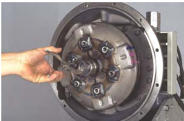
Figure 424 Install bore plug retainer ring.
