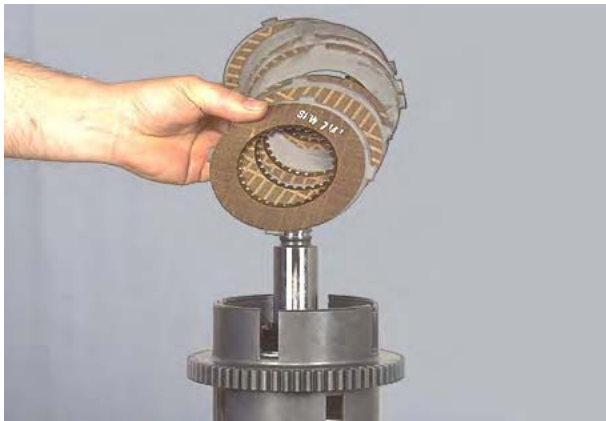
Figure 233 Remove clutch discs.
