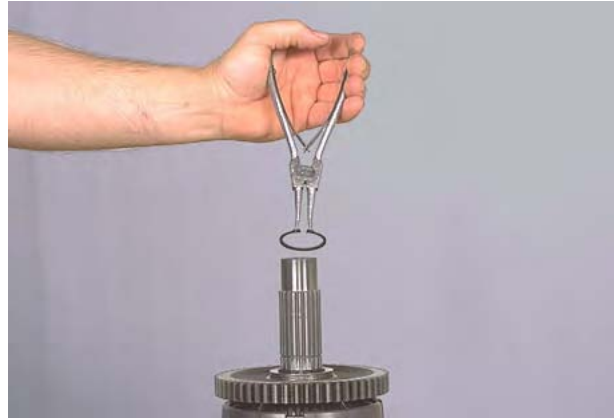
Figure 78 Remove gear locating ring from shaft.
