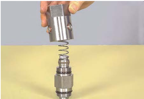
Figure 47 Install inching cover.
