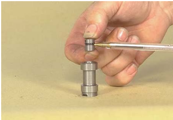
Figure 17 Remove regulator spool sleeve assembly. Remove "O"-ring.
