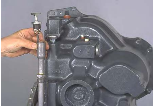
Figure 49 Remove dipstick and dipstick tube.
