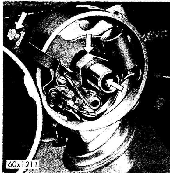
Fig. 50—Distributor Lubrication Points
