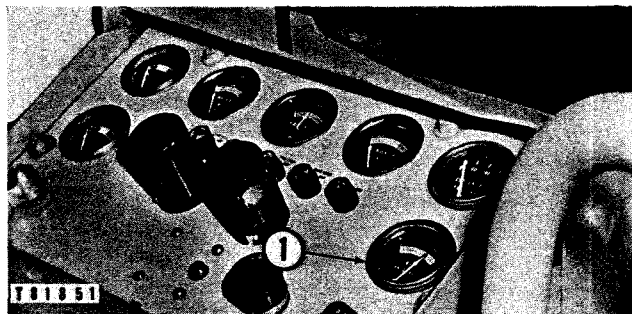
AIR PRESSURE GAUGE LOCATION
