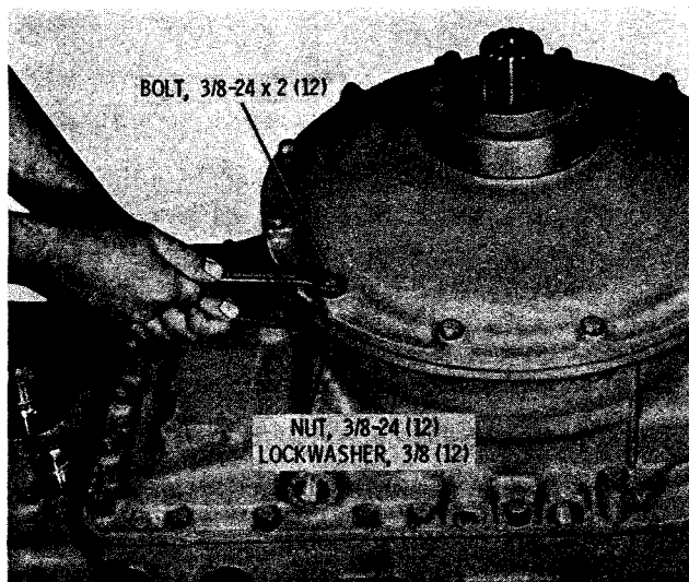
Fig. 7-34. Installing front cover bolts
