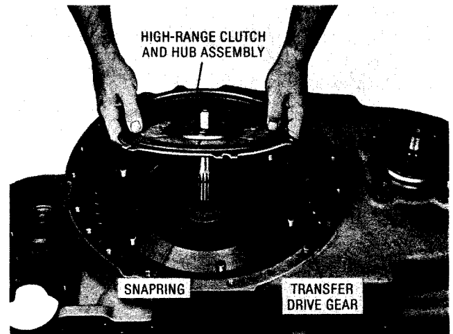
Fig. 7-25. Installing high-range clutch and hub assembly (TT, TTB models without power takeoff)
