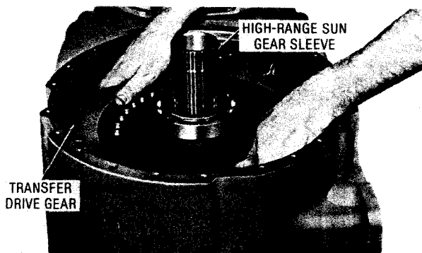
Fig. 5-40. Removing transfer drive gear and sun gear sleeve
