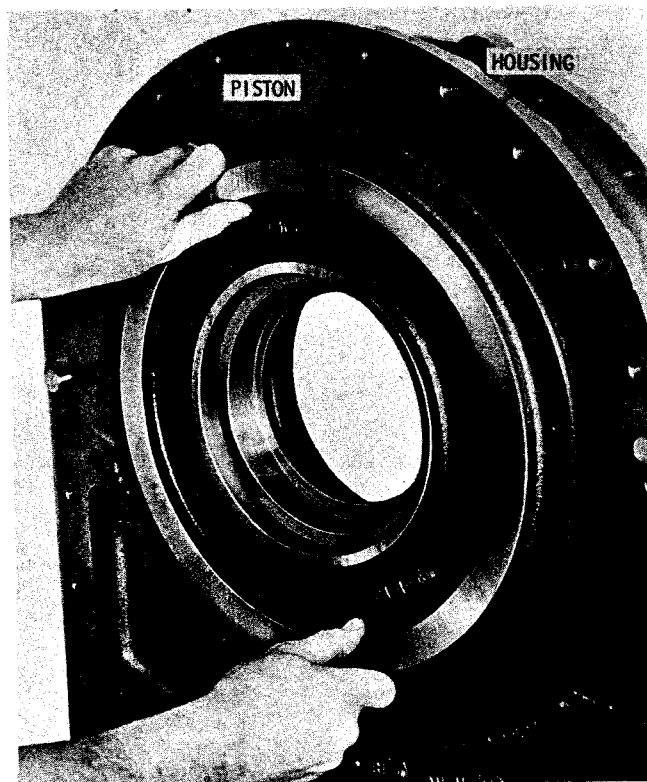
Fig. 7-115. Installing reverse-range clutch piston into transfer gear housing S1751
