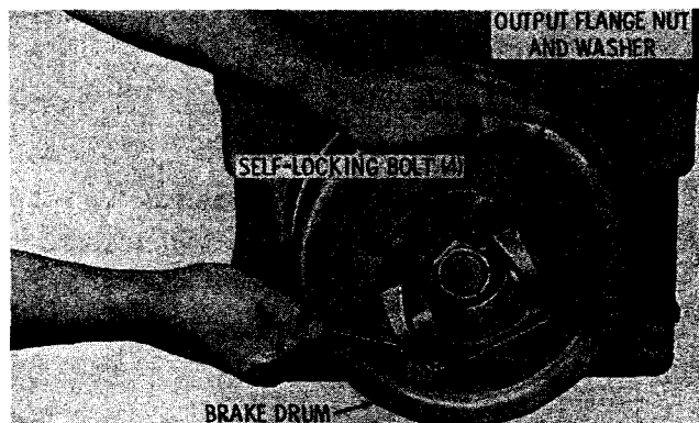
Fig. 5-4. Removing parking brake drum bolts (-1 models)
