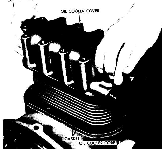
Fig. V-2. Removing (or installing) oil cooler assembly
